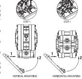
STEP 1 - Slide tab on base assembly (item 23) into desired slot in liquid chamber (item 12).
