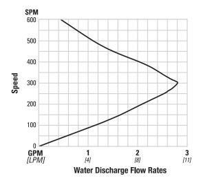
This curve demonstrates the flow created when the stroke rate is varied under static air and fluid pressure conditions. This curve can be applied to different pressure conditions to estimate the change in flow due to stroke rate.
