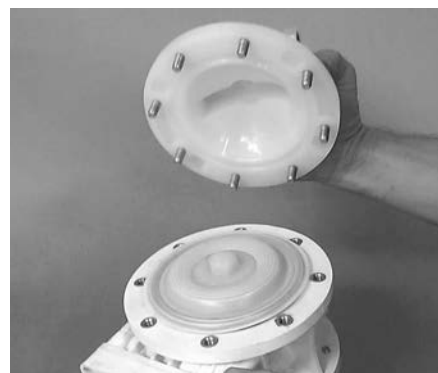
Step 8. Figure 8 The liquid chamber should be removed to expose the diaphragm and outer piston. Rotate center section and remove the opposite liquid chamber.
