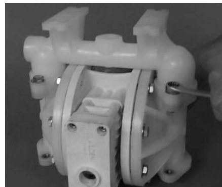
Step 5. Figure 5 Using a 1/2" box wrench, remove the inlet manifold.
