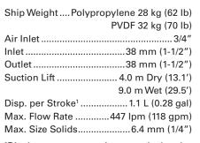
Displacement per stroke was calculated at 4.8 bar (70 psig) air inlet pressure against a 2.1 bar (30 psig) head pressure.
