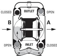
liquid column separated by elastomeric
