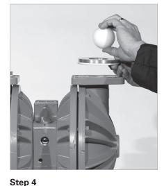
Remove the discharge valve balls
