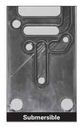
Next, install an optional single-point exhaust gasket (04-2638-52). The single-point air valve gasket can be purchased as a spare part or included with the purchase of a new Pro-Flo® SHIFT pump.
