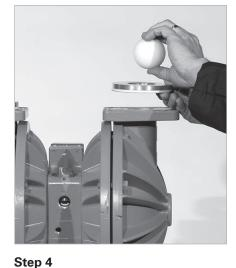
Remove the discharge valve balls
