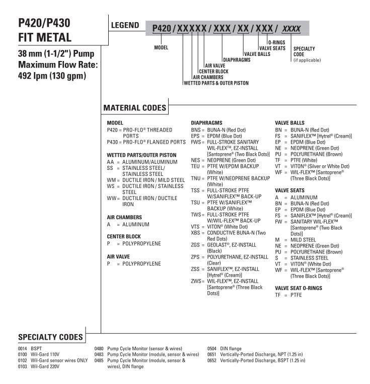
**NOTE:** Most elastomeric materials use colored dots for identification. **NOTE:** Not all models are available with all material options.
