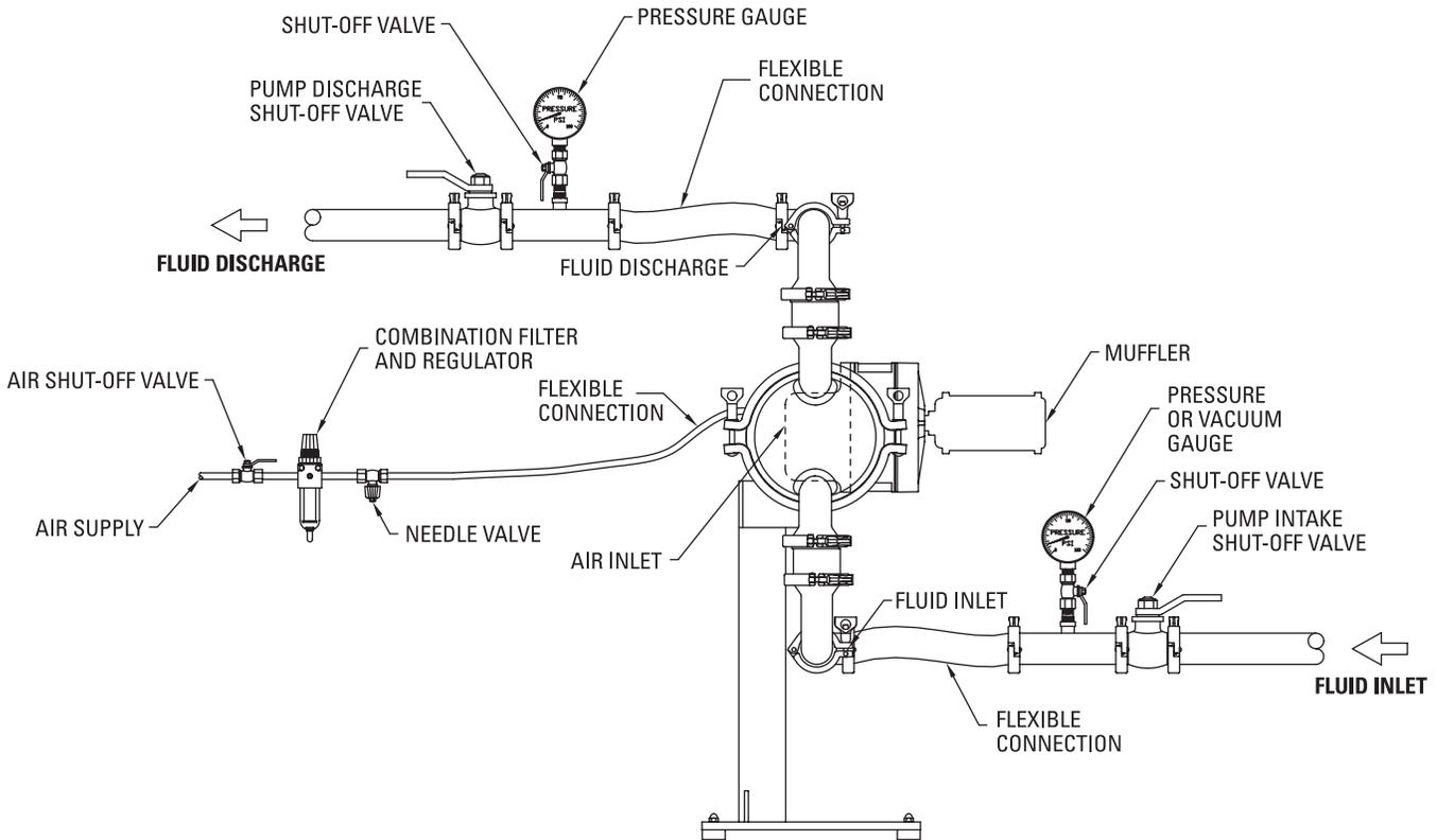
**NOTE:** In the event of a power failure, the air shut-off valve should be closed if restarting of pump is not desirable once power is regained.
