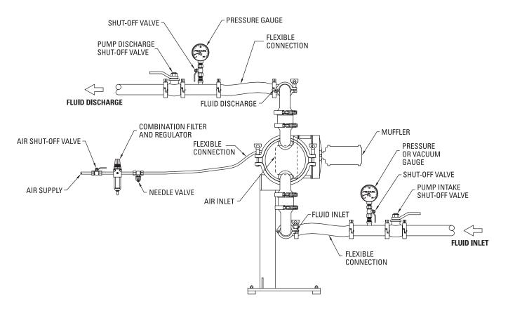
**NOTE**: In the event of a power failure, the air shut-off valve should be closed if restarting of pump is not desirable once power is regained.
